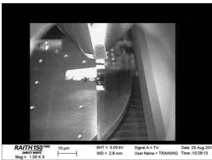
Figure 11 SEM objective lens and sample holder as viewed by the chamber camera
