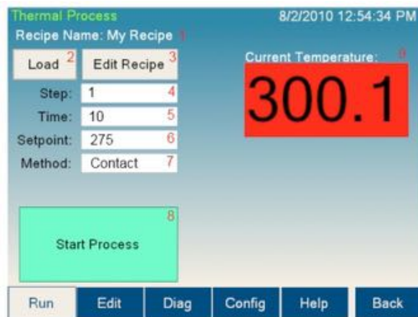
Figure 4: Thermal (Bake) Process Screen
